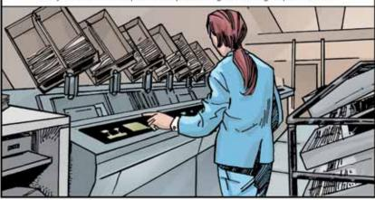
In addition to reading the magnetic ink characters, the processing sorter bundles together all checks drawn on banks in the facility's Federal Reserve District and those drawn on banks located elsewhere. Simultaneously, a computer prints a listing of the checks that were sorted into each pocket and their total dollar value.
